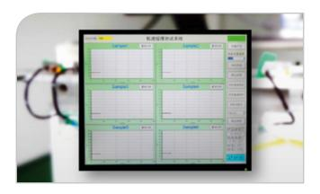
To pass the test, a connection system must demonstrate no significant increase in contact resistance after 20,000 cycles.
