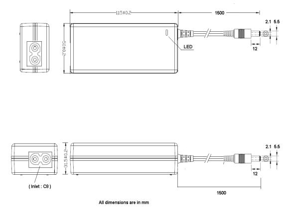
Note: 1. All dimensions in mm. 2. Detail mechanical drawing upon request.
